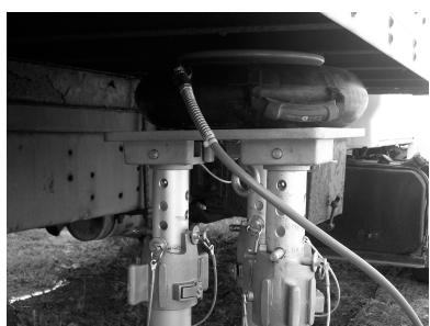
The Prospan system, using various extensions, base plates, and attachments, can be used to support a variety of structures and objects. This section explains how the Prospan system can be used as a column support, a gantry for lifting, and as a stabilization device for vehicles.
