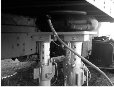
The Prospan system, using various extensions, base plates, and attachments, can be used to support a variety of structures and objects. This section explains how the Prospan system can be used as a column support, a gantry for lifting, and as a stabilization device for vehicles.
