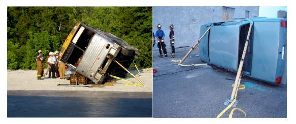
Once initial steps have been accomplished (placement of cribbing, etc.) the installer attaches the telescoping strut to its base plate and then inserts the desired end-attachment.
